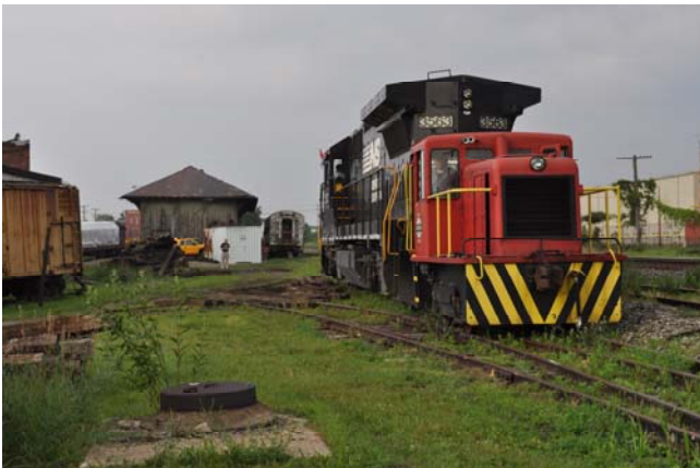
Size comparison between a GE Dash 8 and a GE 25 tonner.
